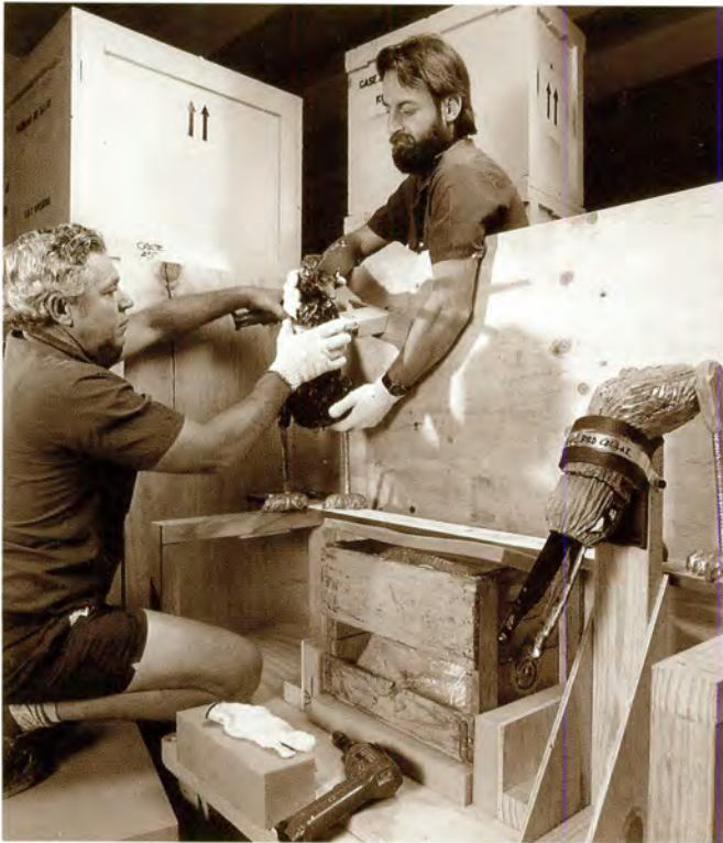
Workshop Co-ordinator Mervyn Brehmer and Artisan Warren Watson constructing one of the specially designed and custom built crates
