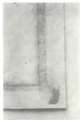
Fig. 3. The narrow stain is made by adhesive tape; the blob at the corner is from rubber cement.
